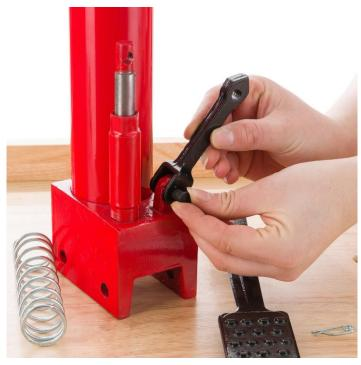
• When tightening, make sure you have enough clearance for the pumping function.
