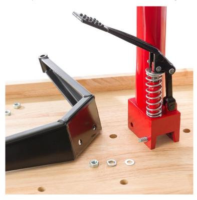
• Fix the base with the foot and tighten the screw connection on both sides.
