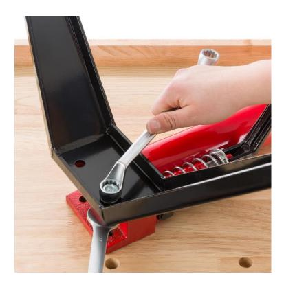
Before attaching the wheels, ensure the vertical position of the shaft to ensure that the transmission jack is secure and that all wheels are touching the level ground securely. Then tighten the screws.
