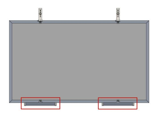
Connect the mounting rail (C) and the 0° support base (E) to the M8x20 screw and tighten them.
