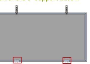
Connect the L-joint (from Part D) to the 0° support base (E) as shown below
