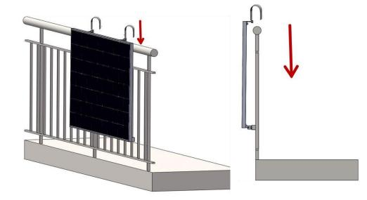
Hang the complete system on the balcony railing, and then fix it with the M8x100 (S2) screw
