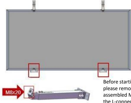
Before starting this step, please remove the preassembled M8x20 bolt from the L-connector on the extension bracket. Put it aside.
