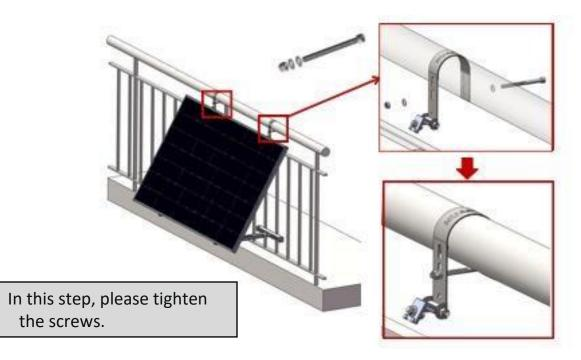
Use an additional rubber pad (F) between the hook and the balcony railing if the gap is loose.
