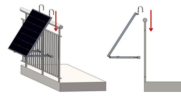
Hang the complete kit on the balcony railing, and then fix it with the M8x100 (S2) bolt.
