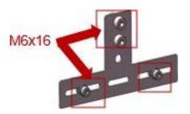
Before starting the assembly, please remove the pre-assembled screw M6x16 from the hook. Set them aside.
