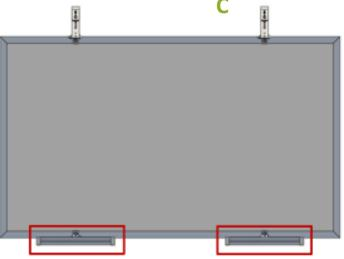
Connect the mounting rail (C) and extension (D) to the outer hexagonal bolt M8x20 (S3) and screw them tightly.
