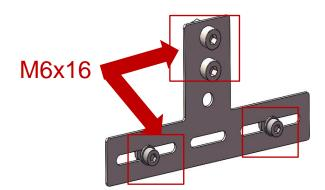
Before starting the assembly, please remove the pre-assembled bolt M6x16 from the hook. Put it aside.
