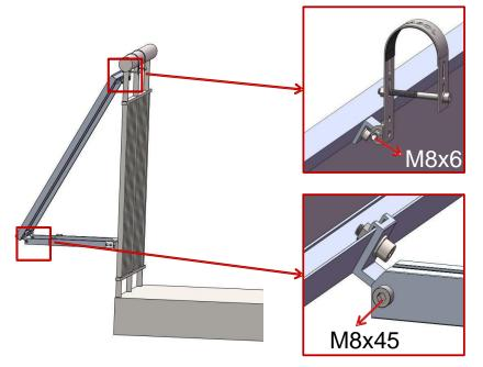
Next, attach the mounting rail (C) to the balcony railing with bolt M8x80 (S2) and tighten it.
