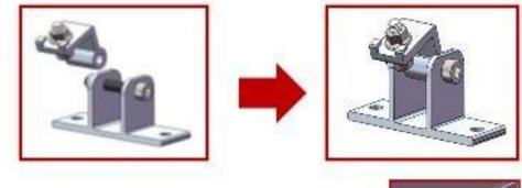
Then mount the base (0°support base with L-joint) on the plate as shown below
