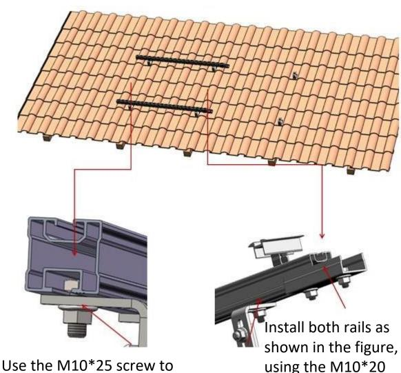
fix the roof hook with the rail
