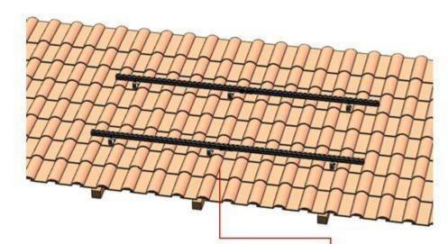
Connect the rails to the M10\*20 bolt and M10 nut as shown in the picture
