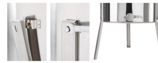
**Step 2:** To install honey gate, remove hex nut (4) from gate piece. Insert gate through the front side hole and secure backside with hex nut (tighten enough to seal O ring).
