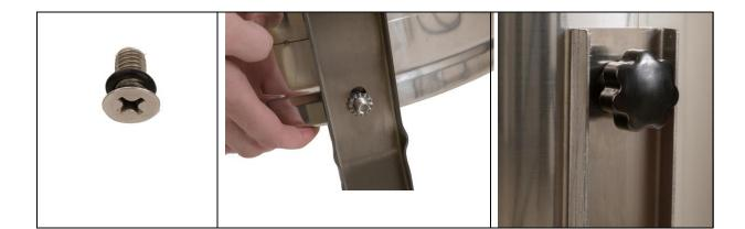
To mount the honey outlet, remove the nut from the outlet piece. Insert the spout into the hole on the front and secure the back with the nut (tight enough to seal the O-ring).
