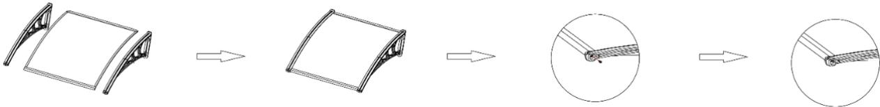
Press brackets on both sides and fix brackets to all four corners with the little screws.
