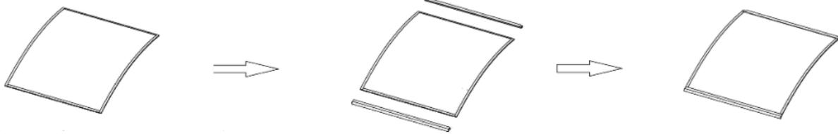
Insert aluminium bars on the two short sides.
