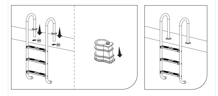
3. After the pool ladder has been completely assembled, cement it at ground level behind the edge of the pool. The placement plays an important role. For wide-spreading or narrowly protruding ladders must be ensured corresponding distance.
