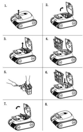
Make sure the power supply is switched off and unplugged.
