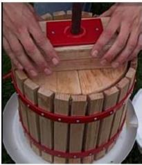
• Place the plastic ring (J) on the printing plate and then mount part (B). Insert the red rod (C) into one of the openings of part (B) and press the fruit by turning it clockwise.
