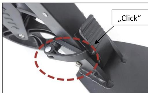
Make sure to fully unfold until you hear the “snap in”. Close the quick release. Make sure it’s tight.
