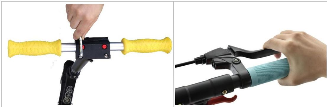
Adjust the lock to tight the T-bar without space, hold the brake handle to restore the brake line.
