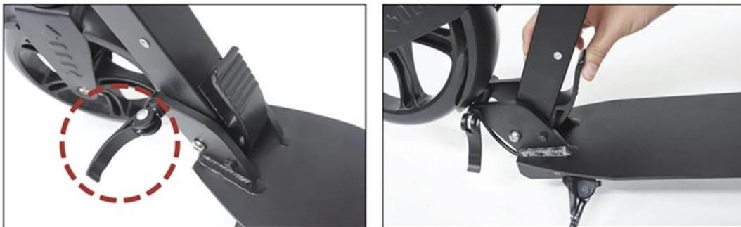
Open the rapid tightening lever and press the folding button to unfold the Scooter.
