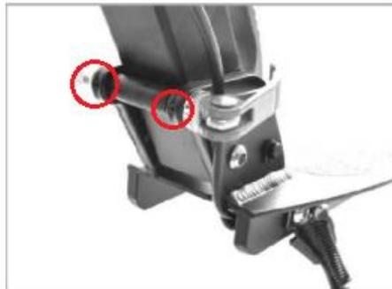
Use the smallest tool to adjust these 2 screws to make the folding tight/loose.
