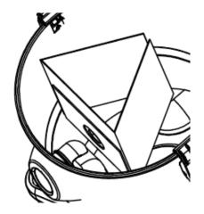
• Attach the top of the vacuum cleaner to the collection container and secure it with the hook.
