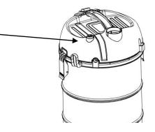
• Release the hook and lift the cover of the vacuum cleaner.
