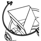
• Attach the top of the vacuum cleaner to the collection container and secure it with the indicated hook.
