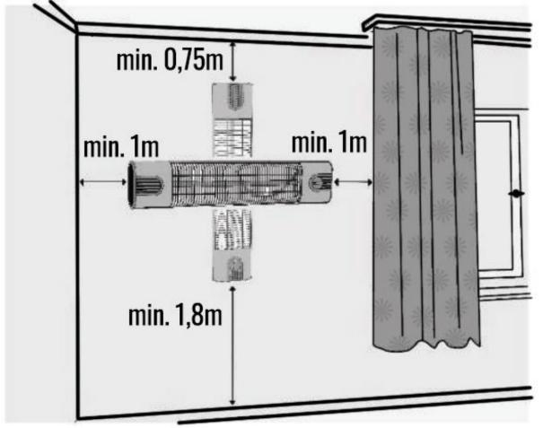
Note: No vertical mounting possible, picture is only for distance clarification!
