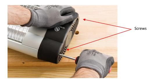
Pull out the endcaps and slide the metal cover to the side.
