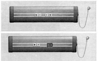
• Fasten the brackets at the appropriate distance of each other (17.7 - 21.7 in (45-55 cm)).
