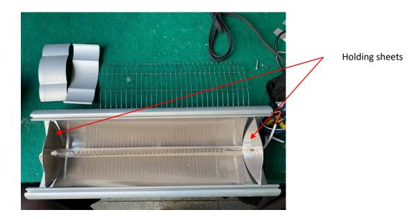
Carefully cut off the cable tie with the cutter. Do not cut the cables! By using pliers remove the blue and red cable from the board. Grab the cable by the very bottom. The lamp is loose now.
