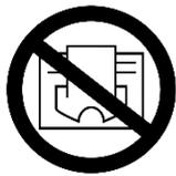
**⚠ WARNING!** The heater must not be covered to avoid overheating and fire hazard!
