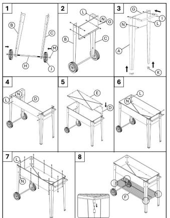
Align the holes in the base plate (E) with those in the skirting boards. Insert screws into each set of holes, starting with the bottom cover. Secure each screw loosely with a nut.
