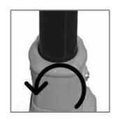
NOTE: Make sure the snap lock remains in place until the steering column is fully extended and securely seated. Before use, check that all parts are stable and safe.
