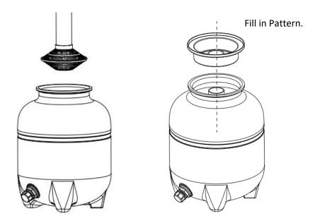
5. ) Fill the tank with sand (max. 20kg). Take away the pattern after filling.
